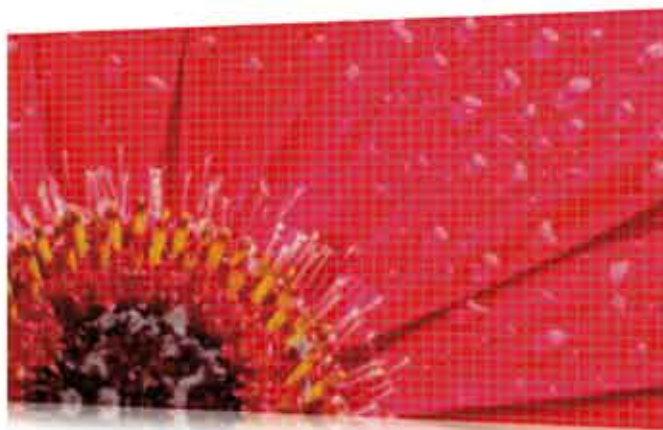
The typical 'screen door' effect seen on projectors without SXRD technology.
