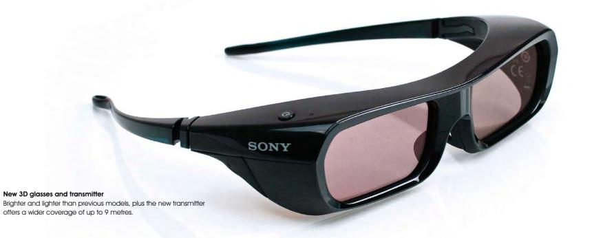
Frame sequential display method with active shutter glasses
